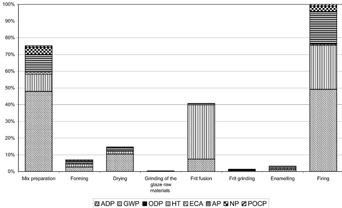
Fig. 9. Ceramic tile — environmental profile of the production operations.
