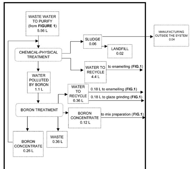
Fig. 2. Ceramic system waste water.
