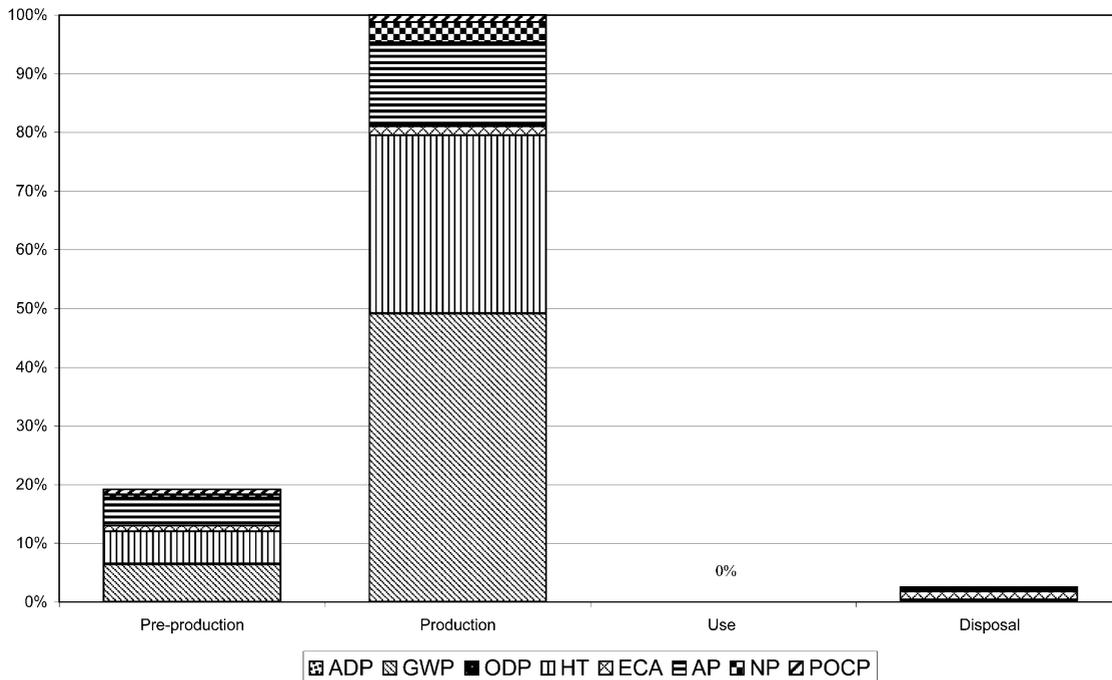
Fig. 6. Ceramic tile — contributions of the life cycle phases to the eco-indicator.
