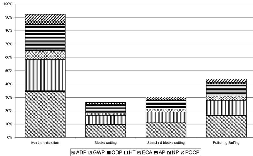
Fig. 10. Marble tile — environmental profile of the extraction and production operations.
